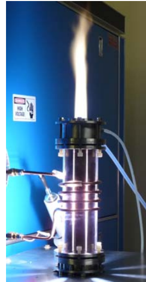
Fig.8. Plasma torch in operation.
